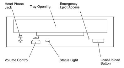
**Note:** Normally the tray makes a ratcheting sound when pulling it open using the above procedure.
